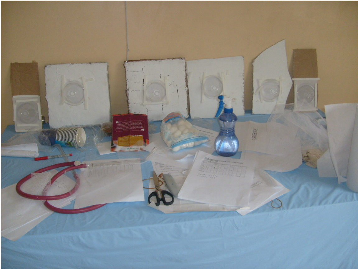
Figure 1 Evaluation of ISONEM SIN-OUT paint on different surfaces in the laboratory. The figure shows WHO test cones attached to treated surfaces arranged thus L-R, negative control, cement, mud, particleboard, asbestos and positive control.
